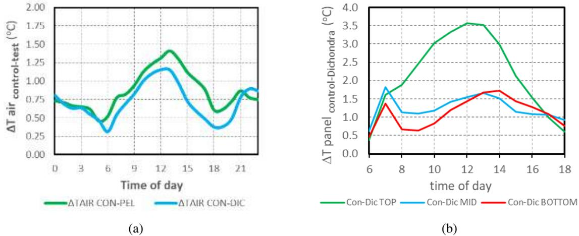
**FIGURE 3:** (a) difference in **air** temperature between control plot and test plots. (b) difference in **panel** temperature between control plot and test plots. In both figures, larger values indicate panels in test plots were cooler. Data for August 2020.
